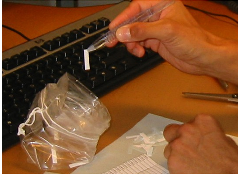
FIG E1. An SAM strip sized 5 × 25 mm cut from a sheet of 8 inches × 10 inches.
